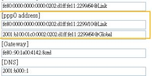
Manually setup the IP address: Select this option to manually set up IPv6 settings if your network environment does not have DHCPv6 server and router advertisements-enabled routers. If you check this item, the following blanks will be displayed for you to enter the corresponding information:
